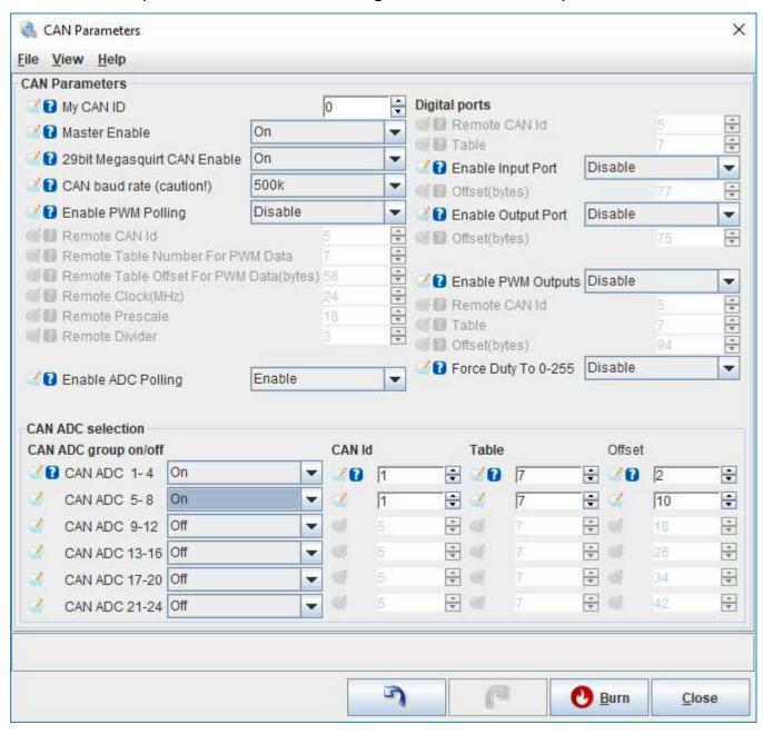
Under the Advanced Engine menu, you can enable thermocouple input under the EGT / Thermocouple Inputs screen. EGT channels 1-8 correspond to CAN ADC01 through CAN ADC08, as shown in the screen below. For Calibration, set Temp at 0V to 32 °F or 0 °C, and Temp at 5V to 2282 °F or 1250 °C. See the appropriate MS3 manual for Actions settings.
