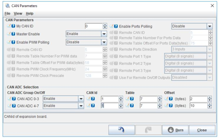
If you have checked the Disable Realtime Data box in the Project Properties to speed up data logging, you will need to download this <u>custom INI file for EGT logging</u> and save it in the ProjectCfg subfolder in your TunerStudio project folder. If you are using the CAN-EGT's LC-2 digital input, you must change the Remote Table Offset for ADC Data number from 2 to 153.
