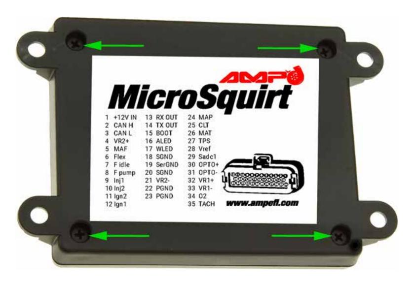
The bottom will easily separate from the MicroSquirt revealing the jumper switch carrier PCB.
