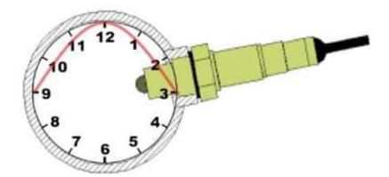
Upright angle: Angle the bung so the sensor elements are at least 10° above horizontal.
