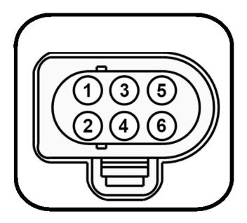
Note: Pin Orientation is shown from **BACK** of connector on the harness side
