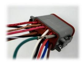
• Ensure the pin is fully seated in the connector, pull back on the wire lightly to ensure the pin has locked into place
