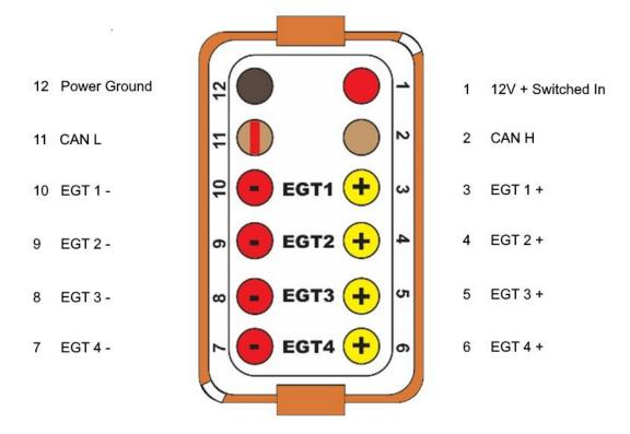
Note: Pin Orientation is shown from **BACK** of connector
