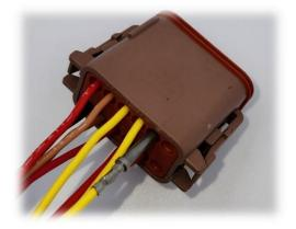
• Ensure the pin is fully seated in the connector, pull back on the wire lightly to ensure the pin has locked into place
