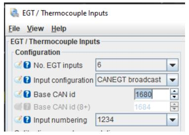
**Starting in FW version 1.6.2** you have the option to select **EGT input numbering.** This is helpful when installing EGT on a V8 engine.
