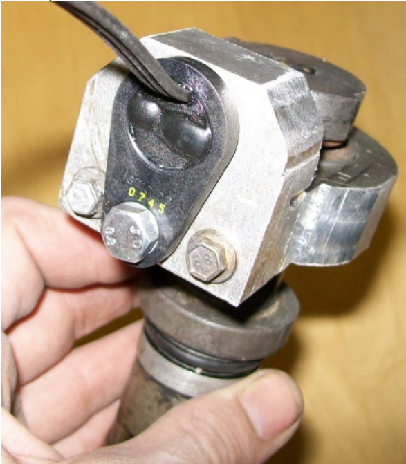
Example of a distributor converted to a cam sensor, using a commonly available gear-tooth sensor.
